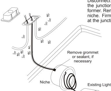
Disconnect the existing light at the junction box or at the transformer. Remove the light from the niche. Firmly pull on the light cord at the junction box and verify that
