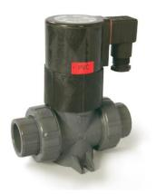
Hayward SV Series Solenoid Valves are true union solenoid valves available in PVC and CPVC. The valves have a corrosion resistant polyester coil and a four-position electrical connection with ½" conduit or SJ type cord electrical connection.
