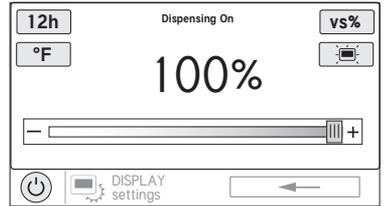
**12/24 hour format** - Toggles between 12 hour and 24 hour time display.
